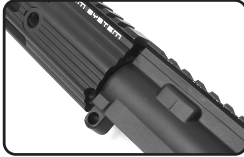
11. With rail offset, line up the grooves on the inside of the rail to align with the teeth on the barrel nut.
