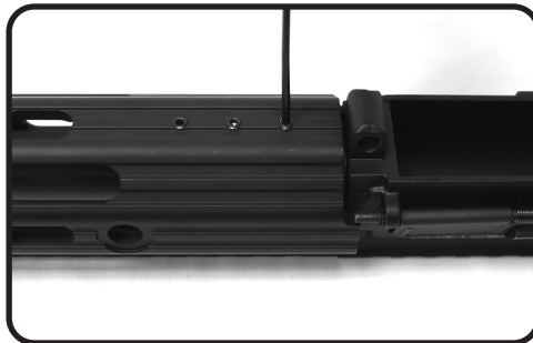
17. Install hex screws on the bottom of RTS. Apply thread locking compound on the three screws.
