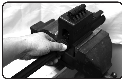
8. Use hand to torque the barrel nut tight to receiver.
