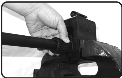
7. Thread the APS barrel nut onto the receiver by hand.
