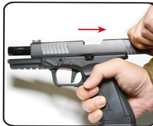
FIRST LOAD & FIRING Pull the slide backward to a specific position, then release the slide forward to load the bullet in the chamber.
