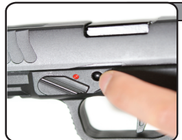
DISASSEMBLY : STEP 2 Push down the pin, from left to right of the slide.
