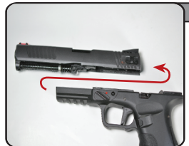
DISASSEMBLY : STEP 3 Pull the slide backward and then push all the way forward until it separated from the receiver.
