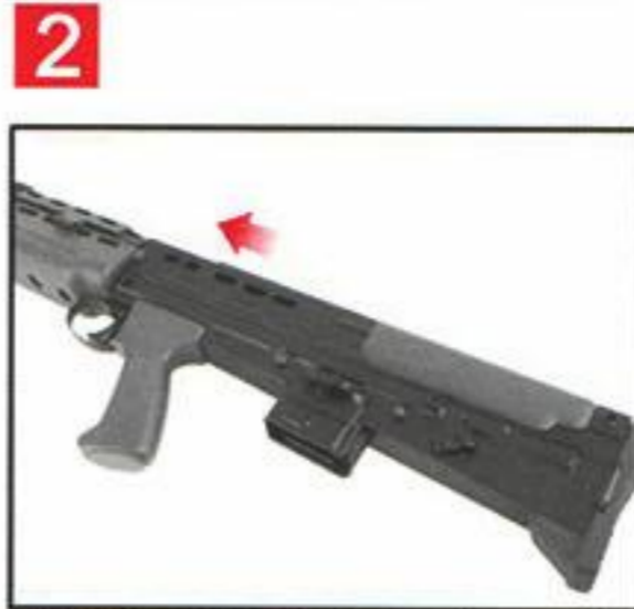
2 Move the upper receiver forward until it is separated from the lower receiver. 移動上接收器，直到它從下接收器分離出來
