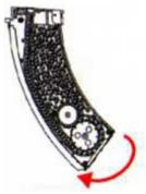
Move the gear with hand clockwise until it is fully wound, and the bullets will be sent up automatcially(It can send about 150 rounds automatically)
