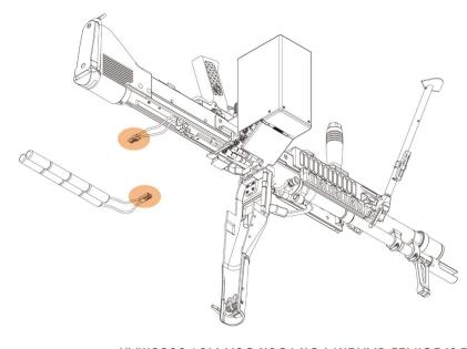
USE THE SPECIFIED BATTERY FOR YOUR GUN 9.6V 3300MAH
