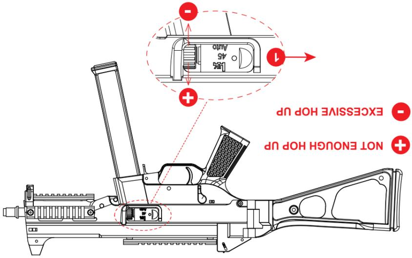
The accuracy of an airsoft gun can be greatly increased by adjusting the hop-up, so you have greater control over where your pellets end up.
