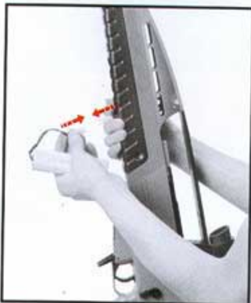
13. Connect the rechargeable battery 连接充电后电池
