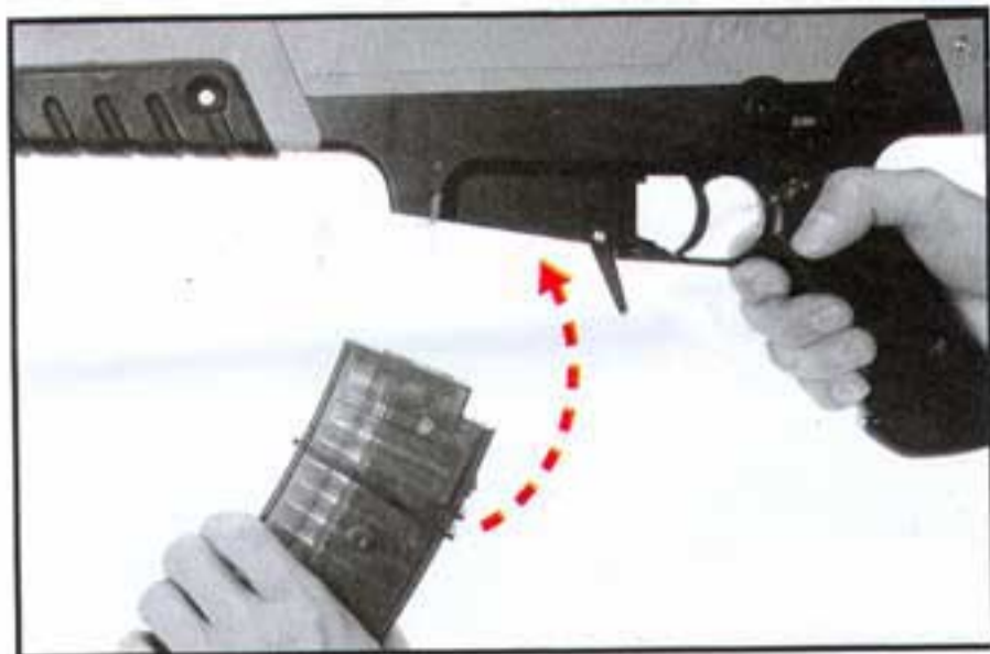
16. Setting the magazine 安装弹仓
