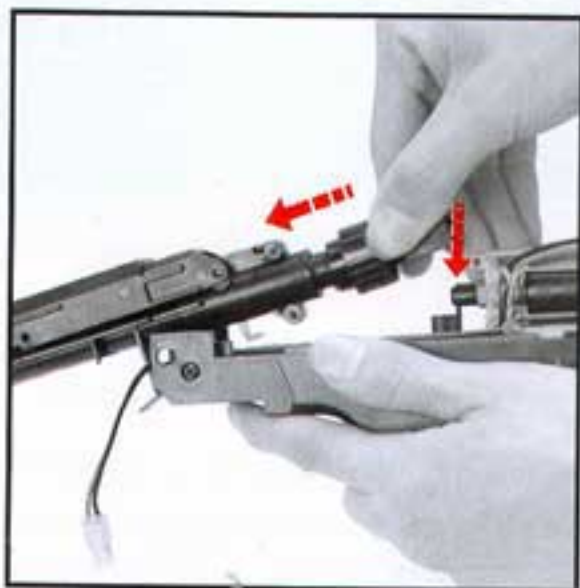
5. Push forward and then down to lock 向前推, 然后向下扣紧
