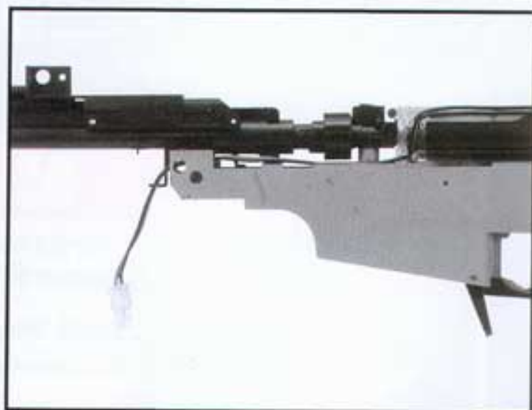
6. Diagram of installed barrel 枪管安装完成图
