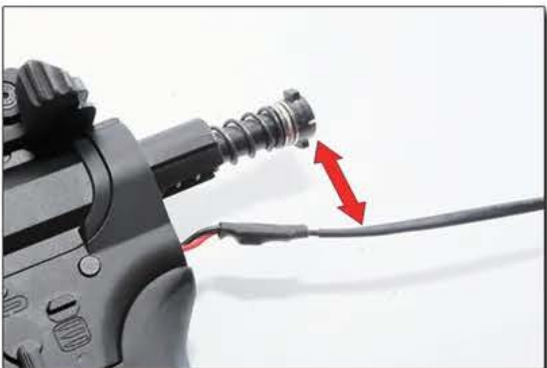
5. Mind the distance between the wire, it may damage the wire due to the rebound.
