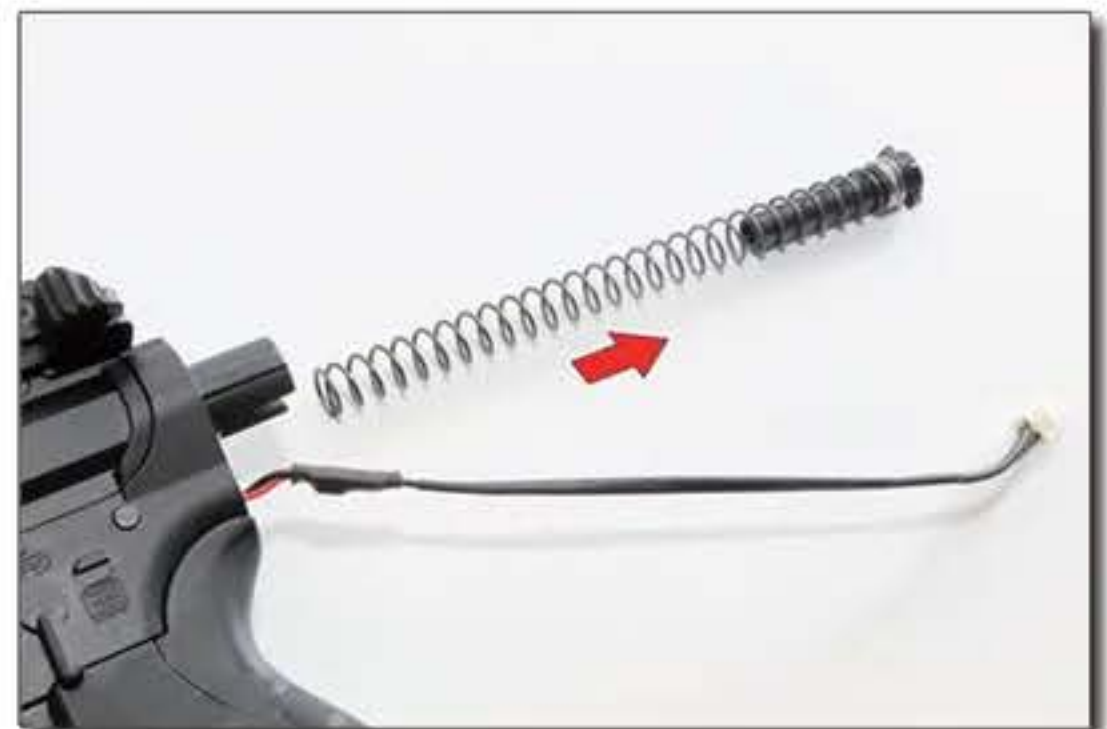
6. Take off the original spring and the spring guide.
