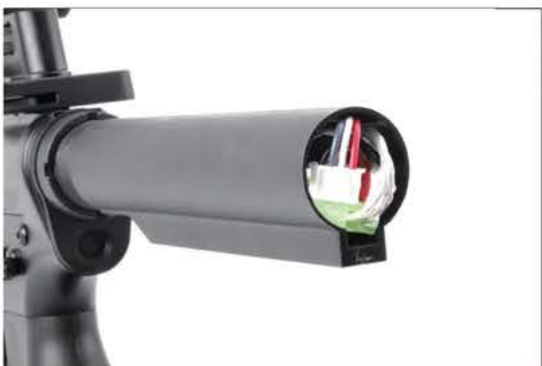
5. Place the plugs and wires back into the pipe.
