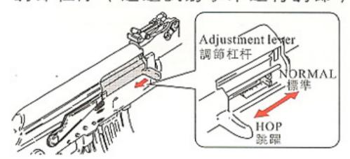
Graduall turn the adjustment dial towards Hop to give hop up to bullets. (The best setting is where bullets fly horizontally.)
