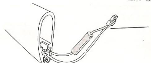
Fuse box (when fuse is replaced, push into the stock all the way.
