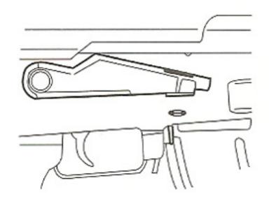
To prevent malfunction of the switch do not change the selector lever from semi to full auto while pulling the trigger.
