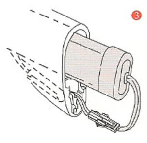
Press down the fuse box and insert connectors and cords between the fuse box and battery. Bend cords in the S shape.
