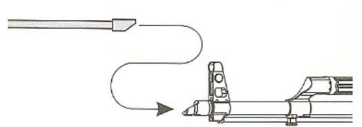
part of the cleaning rod faces down, and remove clogged bullets.
