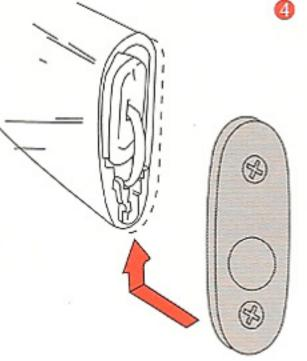
When the battery and cords are set in positions, reinstall the butt plate as shown.
