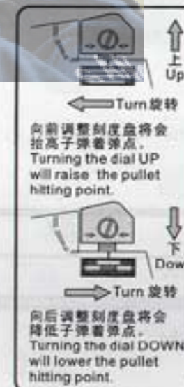
后瞄具3上下调整 Rear Sight 3. For up-down adjustment.
