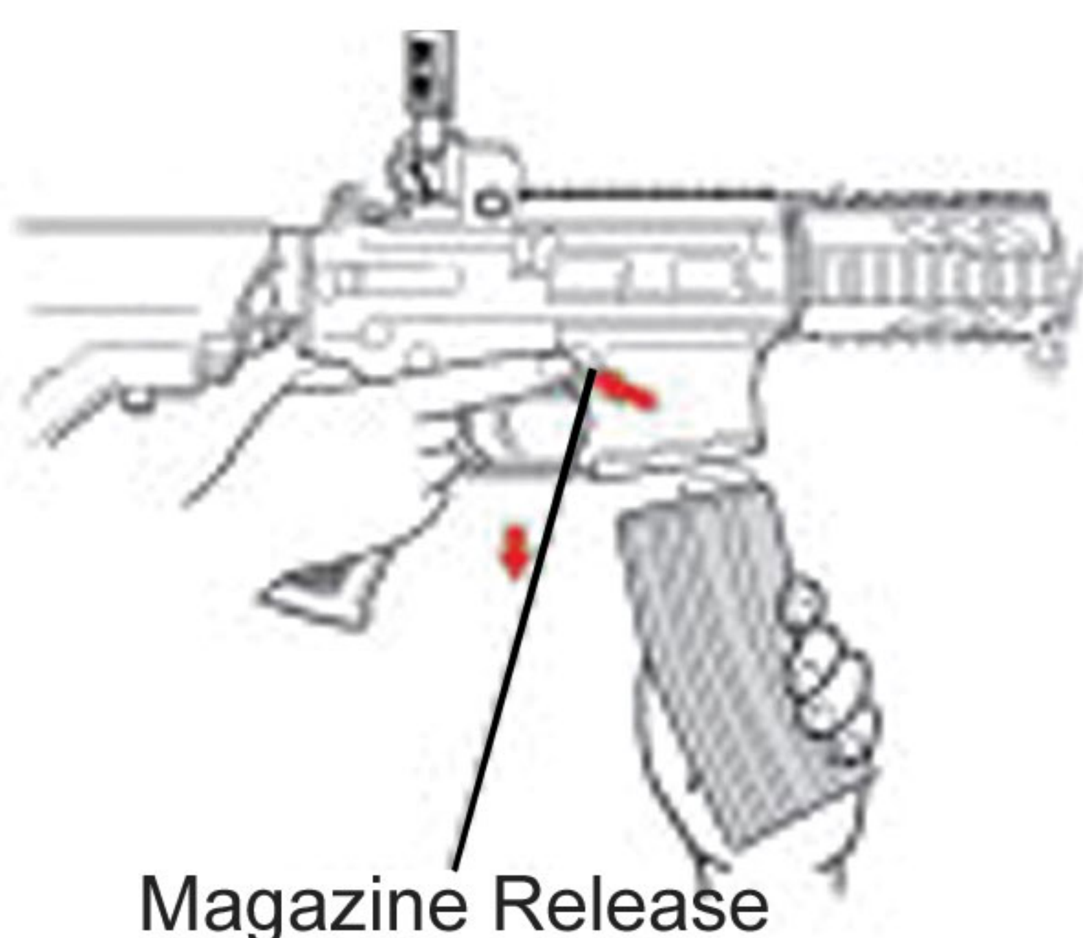
1. Press the magazine release to remove the magazine.
