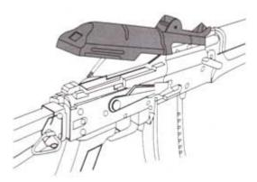
2. Connect the battery to the cord that is accesible from the hole under the rear sight. Press in the battery with its protrusion facing to the left.
