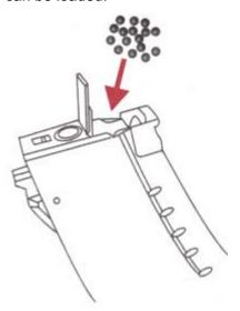
4. Move the gear with hand clockwise until it is fully wound, and the bullets will be sent up automatically. (It can send about 150 rounds automatically.)
