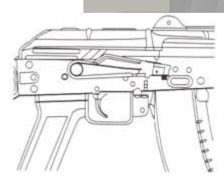
To prevent malfunction of the switch do not change the selector lever from semi to full auto while pulling the trigger.
