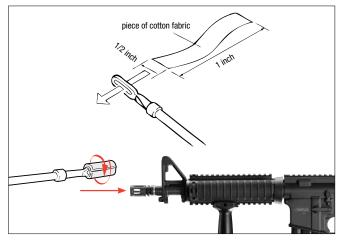
Put the safety ON SAFE and remove the magazine. Prepare a thin rod with a length of approx. 16 inches. Attach a piece of cotton fabric to its end and clean the barrel with some silicone oil.
