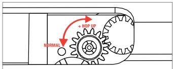
Open bolt to adjust the Hop-Up system.
