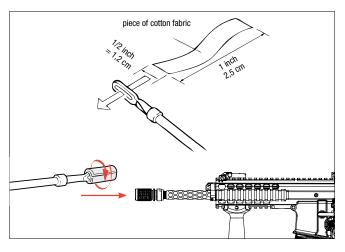
Put the safety ON SAFE and remove the magazine, Prepare a thin rod with a length of approx. 16 inches. Attach a piece of cotton fabric to its end and clean the barrel with some silicone oil. Good care and maintenance of the gun will provide you with many years of pleasant shooting.
