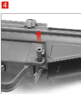
4 Pull the lower receiver locking pin out.
