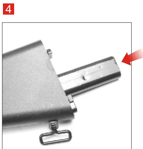
Insert battery into the buttstock.
