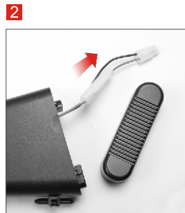
Remove the butt plate and pull out the connector.
