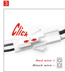
Connect battery plug with the connector.
