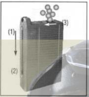
position (2). Open the cover (3) on the top of the magazine and fill the recommended plastic ammo.
