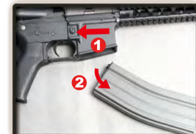
Remove the magazine.
