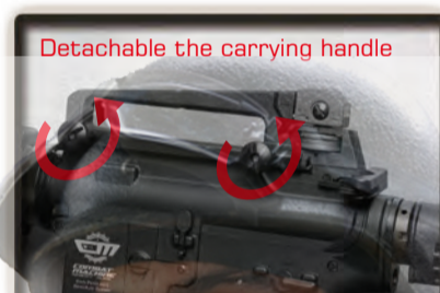
Turn the knobs counterclockwise.
