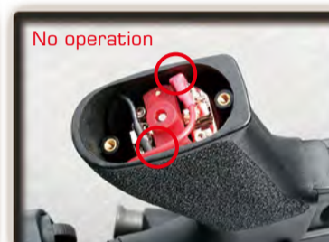
Check the wire set contact with motor.
