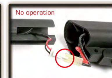
Check the battery and connector.
