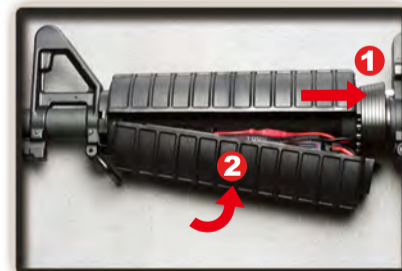
1. Pull the slip ring and hold. 2. Reinstall the lower handguard.
