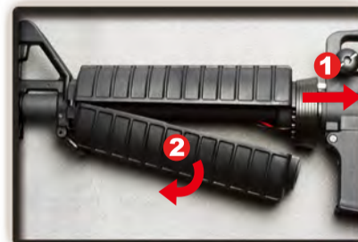
1. Pull the slip ring and hold. 2. Disassemble the lower handguard.
