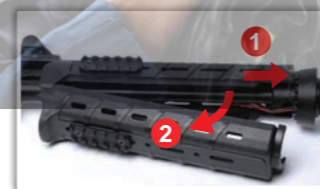
1.Pull the delta ring and hold. 2.Remove the lower handguard.
