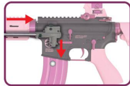
Insert the rod facing down and reaching to the end, and remove clogged pellets.
