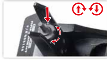
Press the button to adjust front sight up-down. Turning clockwise : Raises the impact point. Turning counterclockwise : Lowers the impact point.
