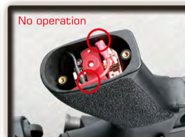
Check the wire set contact with motor.
