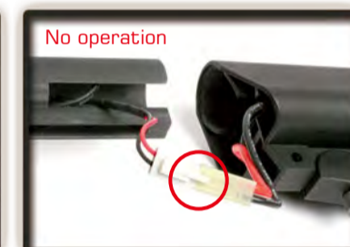
Check the battery and connector.
