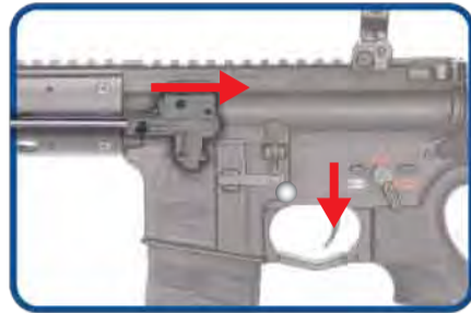
Be aware to have the rod facing down and reaching to the end, and remove clogged pellets.
