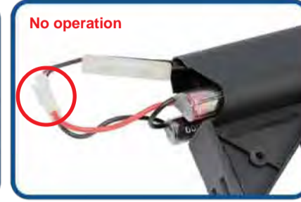
Check the battery and connector.
