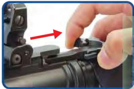
Hold down the button to Pull the Charging Handle.
