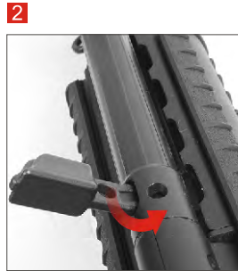
2 Stock the cocking lever to hold the bolt.
