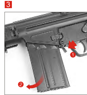
To release the magazine: Hold the magazine, push the magazine release lever and remove the magazine.
