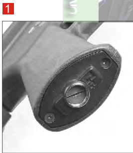
1 The motor adjust screw is at the bottom of the grip.
