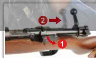
1. Hold the bolt stop. 2. Pull out the bolt from receiver.
