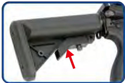
Press the stock release lever to unlock.
