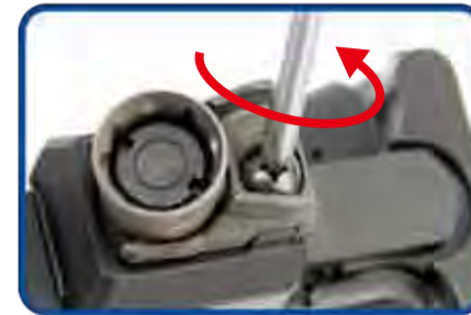
Loosen the rear sight fixing screw and turn the adjusting screw with a screwdriver.
