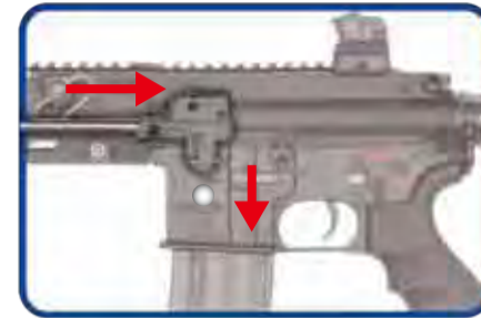
Be aware to have the rod facing down and reaching to the end, and remove clogged pellets.
