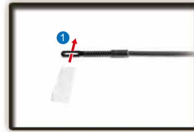
3. Apply a drop of silicone oil or Teflon oil on the cloth and insert the cleaning rod into the inner barrel. 4. Check the cloth and repeat above steps until the cloth can't get any more dirt.
