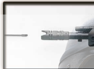
Return the hop up dial to normal position and insert the cleaning rod from the lead edge of the inner barrel.
