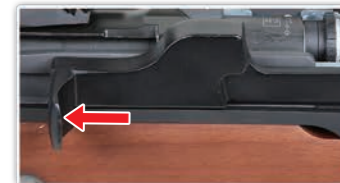
Pulling the bolt handle backward again to release the bolt.
