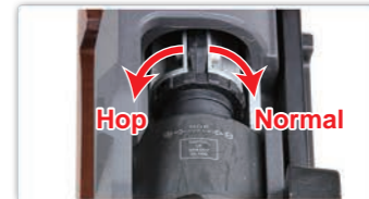
Don't catch your fingers in the dummy bolt. Never hold the gun sideways as the BB pellets will curve right or left.
