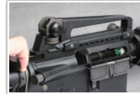
Pulling the charging handle will take the bolt back and open the port cover.
