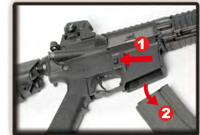
Remove the magazine.
