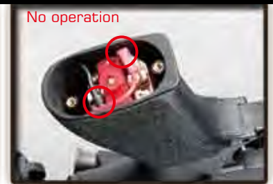
Check the wire set contact with motor.
