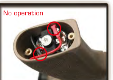
Check the wire set contact with motor.
