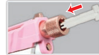
Insert the hopup adjustment tool in the barrel.
