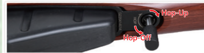
Using hop-up tool to adjust hop by rotating clock or counter clockwise.
