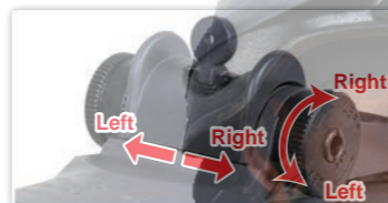
Turning clockwise : Move the rear sight post to the right. Turning counter-clockwise : Move the rear sight post to the left.
