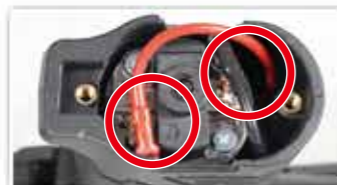
No operation. Check the wire set contact on the motor.
