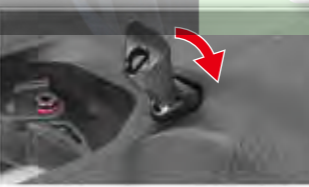
Switch to the other side of the pistol and install the button from the top.
