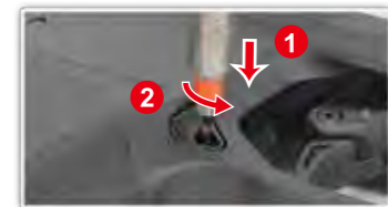
Push down the screw with flat head driver, then turn 90 degree counter clock-wise.
