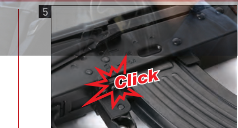
5 Make sure the magazine is securely inserted into the receiver until it clicks.
