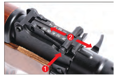
1 Press the button and slide forward or backward for adjustment.
