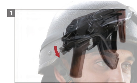
Push the stock lock lever to unlock the folding stock.
