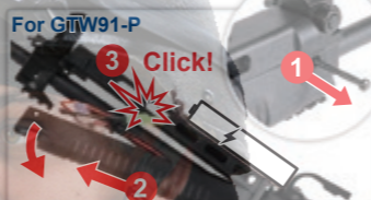
For G&G W91-P 1. Pull out the lower rail pin. 2. Push the lower rail forward and pull up from the back of the lower rail to remove. 3. Connect the battery until it clicks in.
