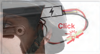
Connect battery until it clicks into place.
