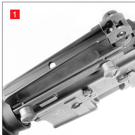
Put on the detachable carrying handle on the upper receiver.
