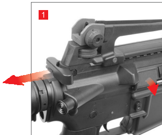
1 Pull the charging handle backward to open the ejection cover.
