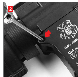
Pull the Receiver pivot pin out. It may be easier to first push the pin hard from the other side of the lower receiver.
