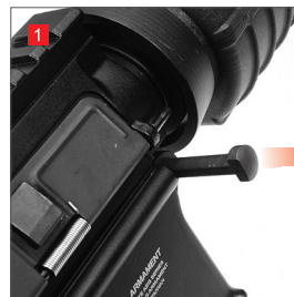
Pull the Receiver pivot pin out. It may be easier to first push the pin hard from the other side of the lower receiver.
