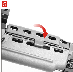
Re-attach left side handguard and close the upper handguard cover.
