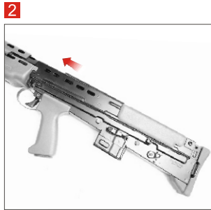
Move the upper receiver forward until it is separated from the lower receiver.
