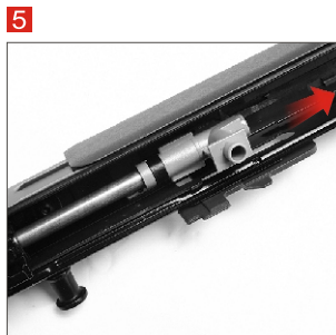
Pull the hop-up unit and inner barrel out.
