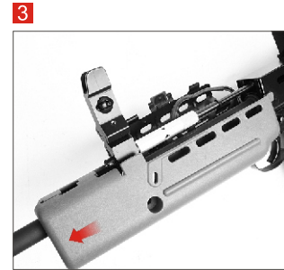
Remove the left side handguard.
