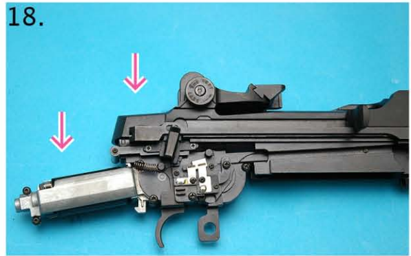
18) 重新安裝馬達 Assemble motor housing into receiver
