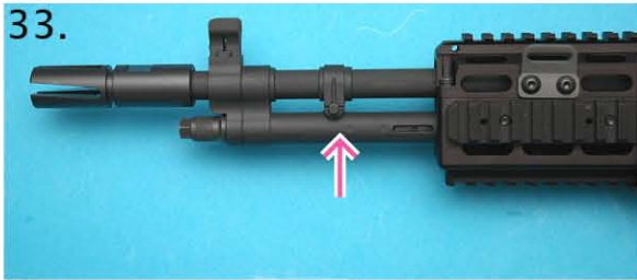
33) 鎖緊準星座 Tighten gas cylinder screw
