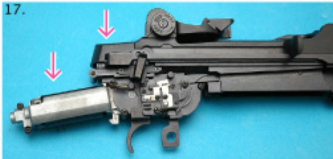
17) 重新安裝馬達 Assemble motor housing into receiver
