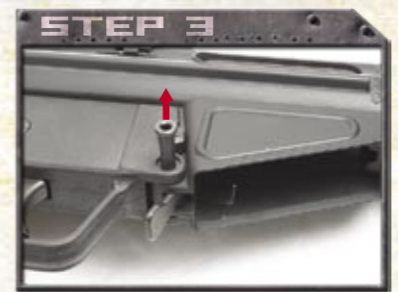
Pull the lower receiver locking pin out.
