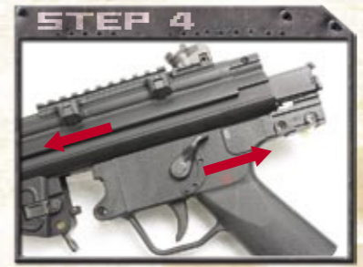
Pull the lower receiver out.
