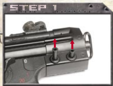
Pull the stock locking pin out.
