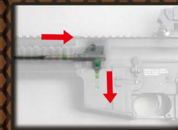
Be aware to have the rod facing down and reaching to the end, and remove clogged pellets.
