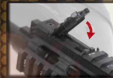
Press against the folding front sight.
