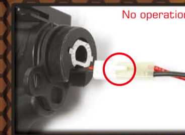
Check the battery and connector.
