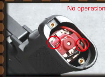
Check the wire set contact with motor.
