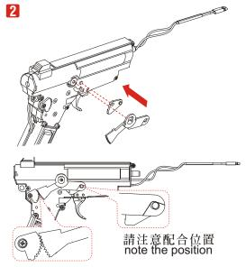
裝入時請注意齒片配合位置 note the gear wheel position while assembling
