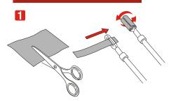
將棉布剪成長約25~30mm 寬約10mm後再捲繞在通槍條上 Cut the cotton cloth length: approx 25~30mm / Width approx:10mm and wind the cut cotton cloth
