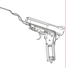
請將電線依圖示做好整理 Arrange the wires as pictured above.
