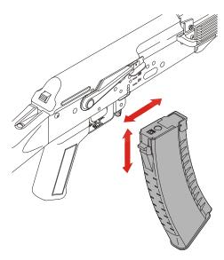
按下彈匣卡榫即可將彈匣裝入或拆下。 Press the magazine release lever to load or unload the magazine.
