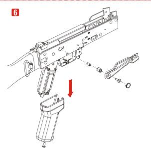
卸下選擇桿及選擇桿連動軸套握把等零件 Remove the fire mode selector lever and grip.
