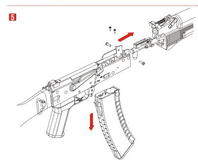
旋開槍管座螺絲 , 將前槍身往前推 , 再卸下彈夾 Loosen the reinforced outer barrel screw. push forwards the rear sight set and remove the magazine.
