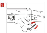
以六角板手將馬達齒輪間隙調整到最佳位置,請勿自行調整。 Use a hexagonal allen wrench to fine tune the engagement between the motor and bevel gear. Don't adjust by yourself.
