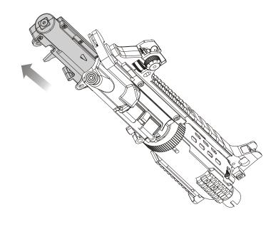
**▼-2** Remove the lower Gearbox 下槍身拆卸
