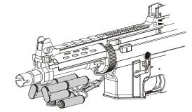
②將電池裝入接上電線 Insert the battery under the barrel and connect the battery.
