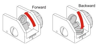
近距 將覘孔往前推 Common/close-range/ low-light shooting. Push forward to engage battle sight. 遠距 將覘孔往後推 Precision daylight shooting. Push backward to engage peep hole.
