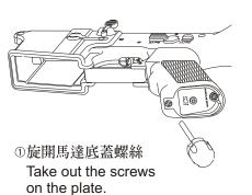
②將馬達拆下 Take the motor out.
