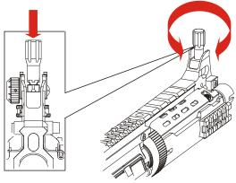
將準星調整桿壓入定位轉動即可調整高低 Turn clockwise to raise B.B. hitting point. Turn counter clockwise to lower B.B. hitting point.
