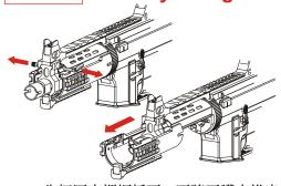
①先把固定螺帽拆下,再將下護木推出 Release 2 pins can Remove the lower handguard
