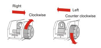
依旋鈕方向旋轉即可將覘孔組左右調整 Trun clockwise to aim right. Turn counter clockwise to aim left.
