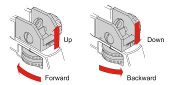
將調整鈕往前轉即可昇高覘孔組, 將調整鈕往後轉即可降低覘孔組。 Turn the dial forward to raise the hitting point. Turn the dial backward to lower the hitting point.
