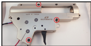
19. Secure the gearbox by 3 screws for microswitch testing.
