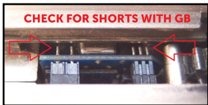
18. Check if the top board fits in the gearbox without any problems.
